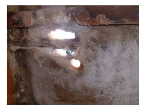
It had a large amount resin putty between the stays and the holes/slots cut into transom and some squished into the area covered by the circular external plate.
