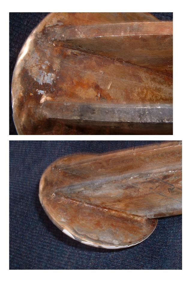
While I like the idea of using the external circle to carry some load due to all the rot in the rest of the system mine was responsible for all the load. I don't think the welds would take it as they looked like fine light duty welds you might see on a bimini or dodger frame. They need to be structural welds not just cosmetic welds.
