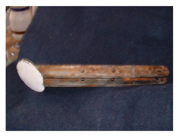
IMHO, the welding is inadequate as the welds (TIG) are only on the outside portion of the plate/stay junction, not on the inside, are very small or thin and do not look to have penetrated much at all.
