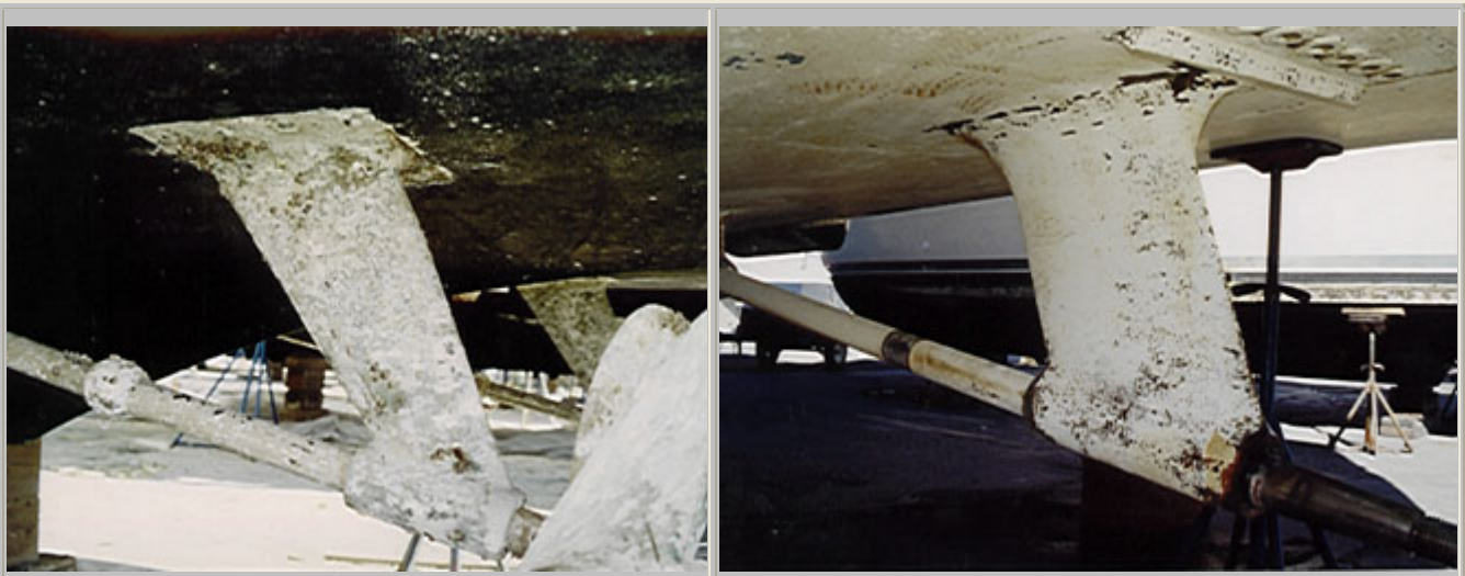
LEFT: There's no way this long, thin strut is going to prevent the propeller from fluttering and causing vibration. The shaft is also too long and extends beyond the strut by 3". Distance between strut and prop hub should be no more than 50% of shaft diameter. RIGHT: Both these boats have the same size propeller. The strut on this Hatteras is three times larger with a mount base the same width as the strut length.
