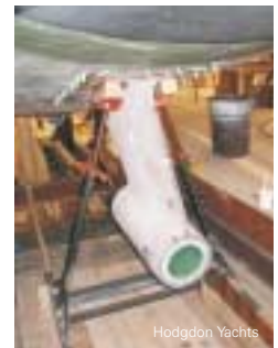
Scheherazade's propeller shaft strut before it was attached to the hull. The strut was built of carbon fiber by Goetz Marine Technologies.
