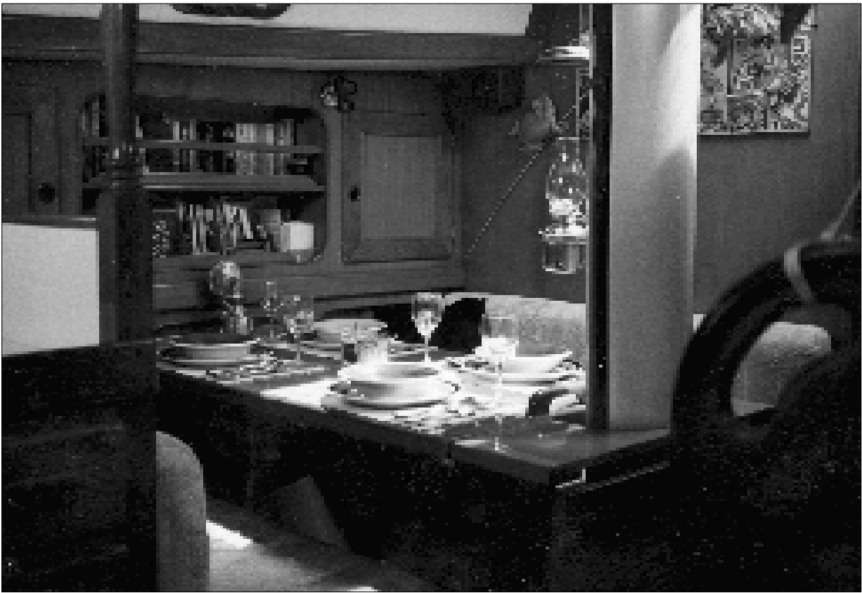
The P-44's main saloon is, unfortunately, dominated by the presence of the mast running right through the dinette table. But it's a "feature" you get used to that provides a good handhold in rough weather and a good place to fix a kerosene lamp. Across the way, the starboard settee makes a great seaberth.
