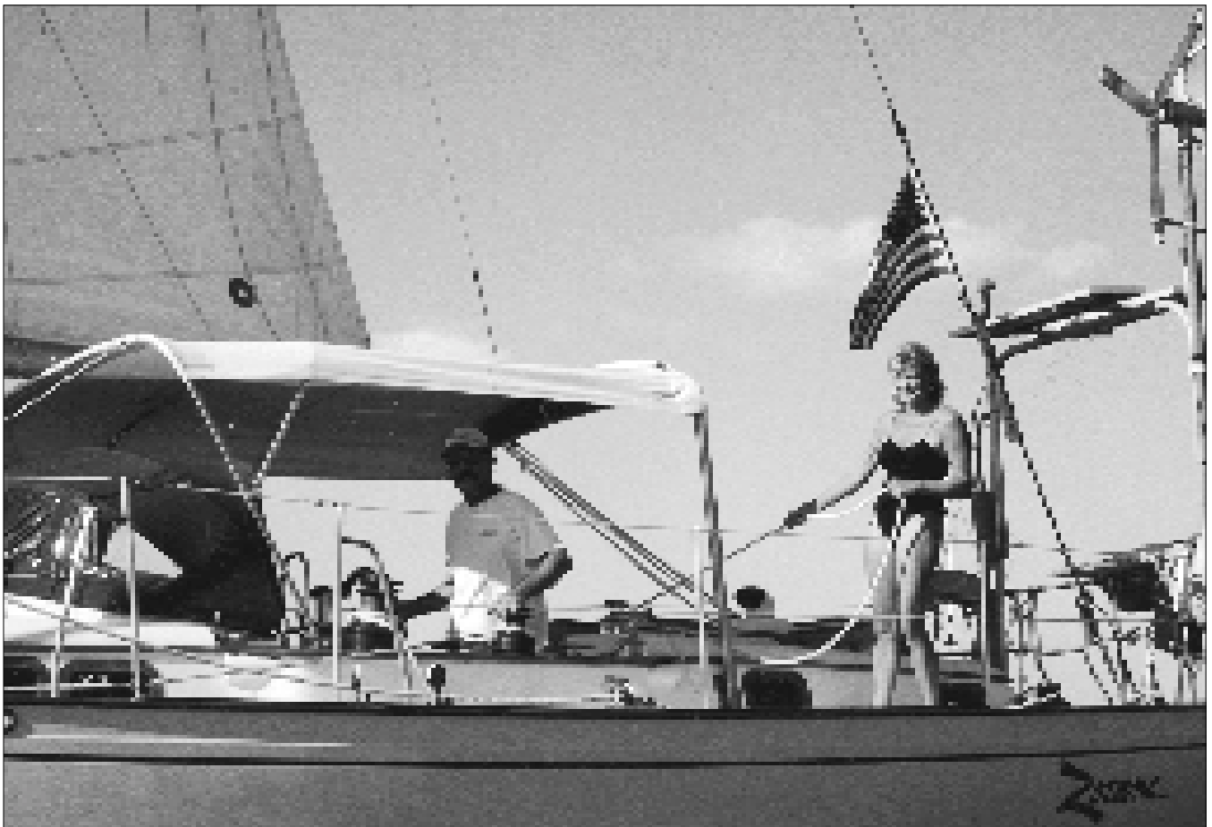
The semi-permanent bimini over the center cockpit, attached at the aft end to the boom gallows, provides plenty of sun protection. The nicely bowed dodger is strong enough to stand up to bad weather and keeps spray and rain out of the companionway. The Windbugger, solar panels and antennas are mounted on the simple arch on the afterdeck.
