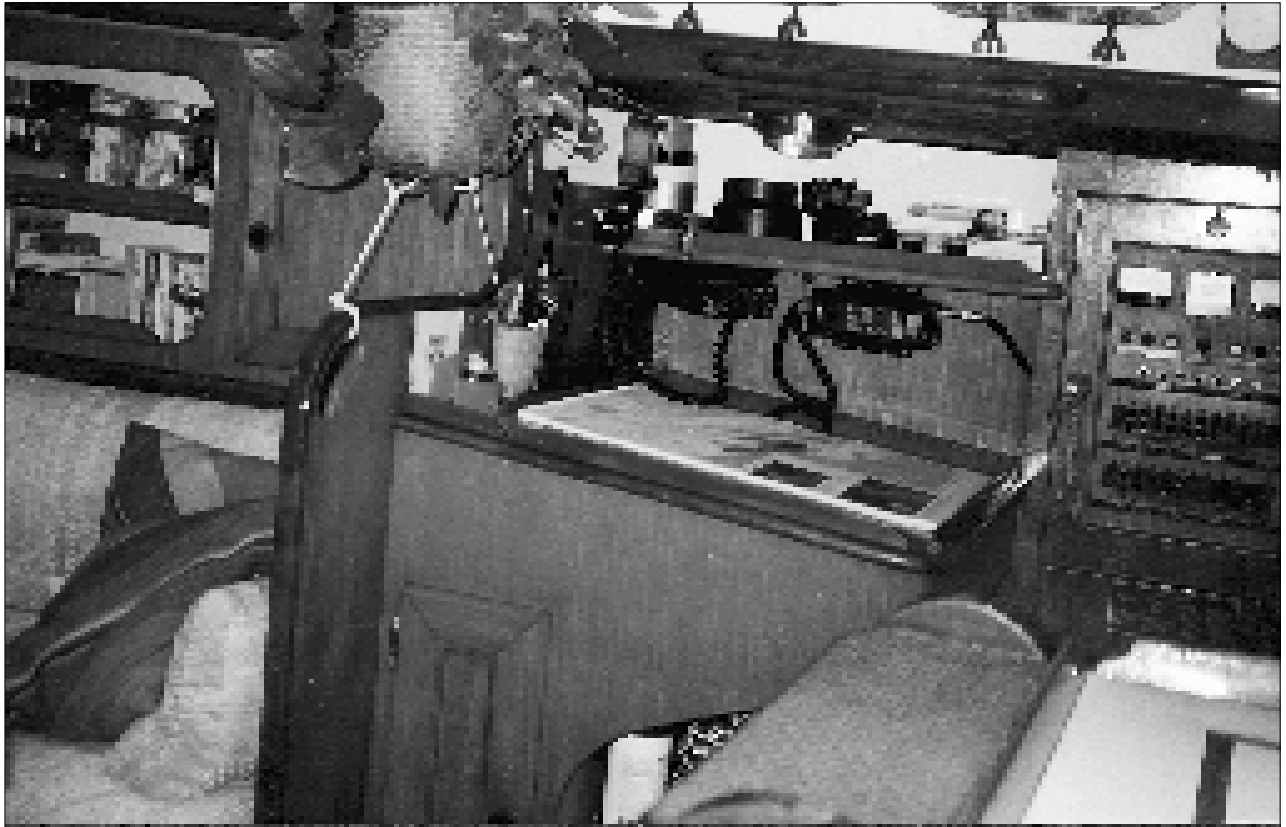
The chart table, to starboard as you descend the companionway, is large and comfortable. The table will take a chart folded in half. There is limited room above the table for electronics, particularly if you want a CRT radar, and not a lot of space for books, tables and guides. The main breaker panel is next to the navigator's seat.
