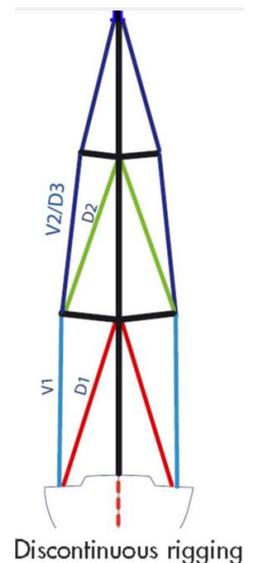
*Beatrix* originally came with Discontinuous Rigging, which is the preferred design. Continuous Rigging is only favored when less expense and ease of installation are important, as they are to a cost-saving boat-builder. Many of the Peterson Cutters have a Continuous Rig. If you are in the process of re-rigging from scratch, I would recommend shifting to the Discontinuous design.
